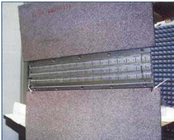
Figure 9, (right): Test jig for subarray measurements consisting of three T/R modules
