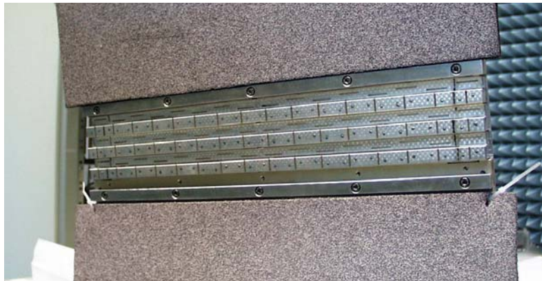
Fig. 5: Setup for an array consisting of three T/R modules
