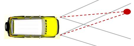
The two antennas can be spaced closer, e.g.  $\lambda/2$  free space distance apart to allow direction of arrival (DOA) estimation of a target detected by the radar.
