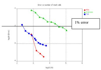
Fig. 3. Error of the line impedance of a coaxial cable vs the number of mesh cells.
