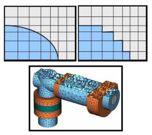
Fig. 2. Examples of PBA, staircase and tetrahedral meshes.
